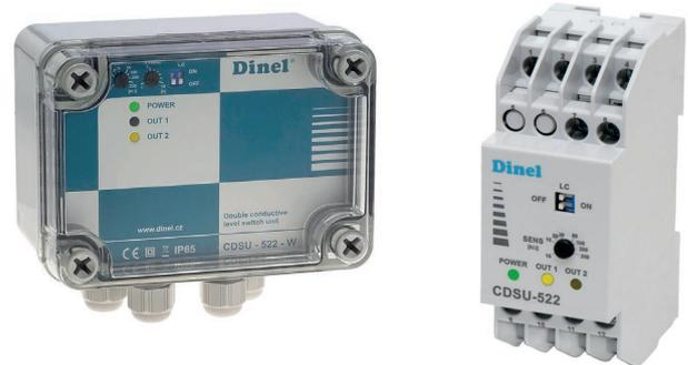
**Level control relay CDSU** are dual channel units designed to evaluate the states of the conductive probes. They include power supply 5 V AC for supplying the probes. The DIP switches enable to select a basic mode (an independent function of two limit sensors) or the level control mode between the maximum and minimum level (pump control). The level control relay allows continuous sensitivity adjustment and time delay set up by trimmer.
