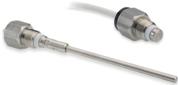
Conductive probes CNP-18 are designed for direct detection of conductive liquids level (water, water solutions). The process connection is M18x1.5 threaded connection, and electrical by fixed cable or screw connector. The probes are connected to Dinel evaluation unit, type CDSU-522 (CDSU-522-W), or other types of evaluation units suitable for connection of the conductive sensors.
