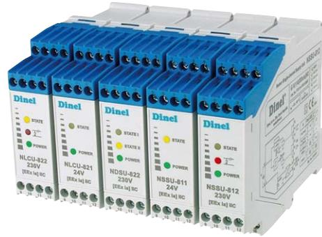
Supply and switching units NxxU are used for energizing of NAMUR output sensors (DLS–27Xi, CPS–24Xi etc.) located in hazardous explosive areas. Due to state of connected sensor they switch their output changeover relay contact or transistor switch. Moreover they can provide simple 2-state level regulation (pump-up and pump-down control).
