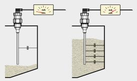
Measurement of electrically non-conductive materials:
