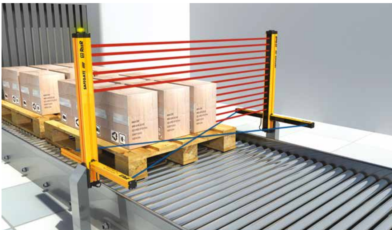
Palletizer with regular pallets transit showing a Safegate with MA Muting arms (integrated sensors)
