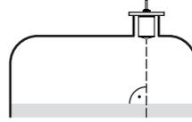
Fig. 16: Alignment in liquids
