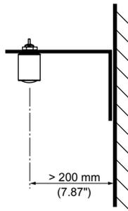
Fig. 7: Mounting via a mounting bracket
