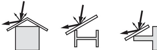
Fig. 15: Cover flat, large-area profiles with deflectors
