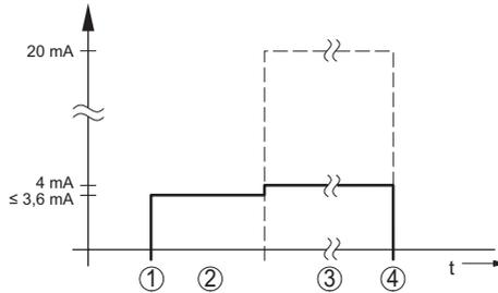
Fig. 3: Run-up time and measured value output
