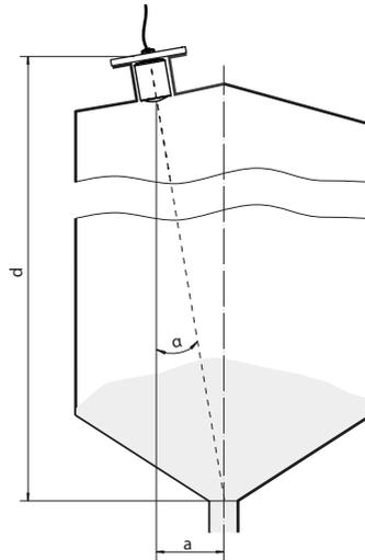
Fig. 18: Proposal for installation after orientation NivoRadar 4100
