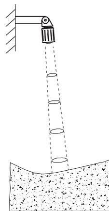
Aiming of the antenna to the center of the silo allows measurement down to the bottom
