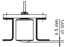
Fig. 13: Recommended socket mounting of NivoRadar 4100
