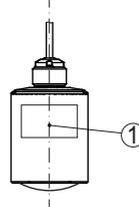
Fig. 8: Position of the polarisation
