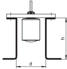
Fig. 14: Socket mounting with deviating socket dimensions
