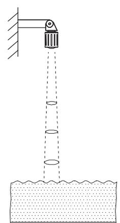
Vertical installation without aiming of the antenna
